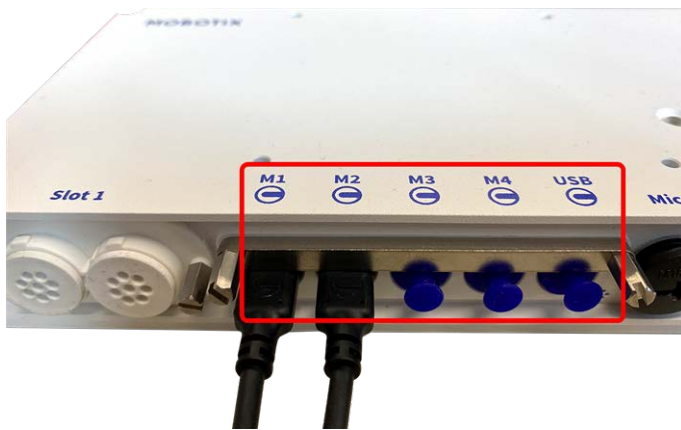
Fig. 22: 4 Module Connector Ports and 1 USB-C interface
