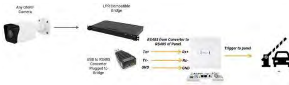
Figure 117. Connection between the Mobotix Bridge to the Brivo Panel using an USB to RS485 converter
