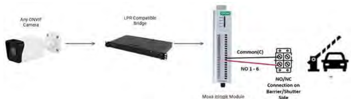
Figure 121. Moxa Connection to a Barrier/Shutter
