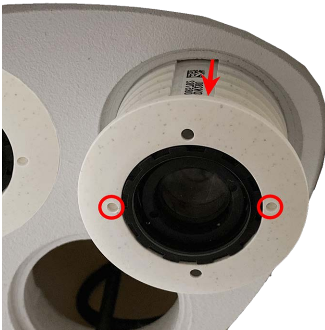
Fig. 10: Remove sensor module from the module housing
