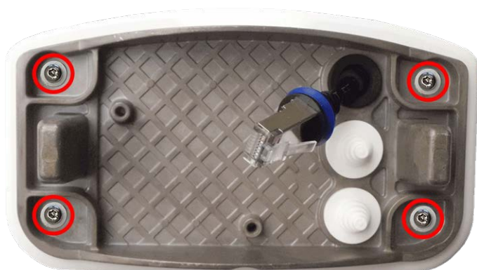
Fig. 6: Installed and ready for Connector Box RJ45
