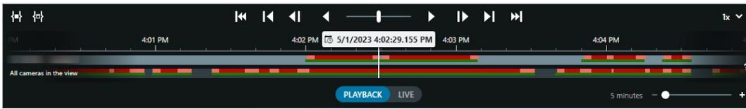
The main timeline displays an overview of time periods with recordings from cameras and other devices in your current view. The main timeline is available on the views tabs and has various controls you can use to navigate your recordings during investigations or to select recording sequences for export, protection with evidence locks, addition of bookmarks, or other.
