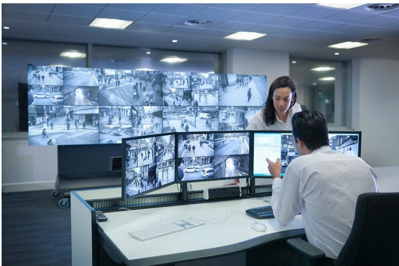
MOBOTIX HUB Video Wall allows operators to view static video walls as defined by their system administrator with a fixed set of cameras and monitor layout. However, the video wall is also operator-driven in the sense that operators can control what is being displayed. This includes:
