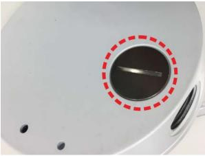
3. Place the camera at the installation location. Mark the position of the two screw holes and the back conduit entry (for cable entry use) indicated in the right figure on the ceiling or wall.
