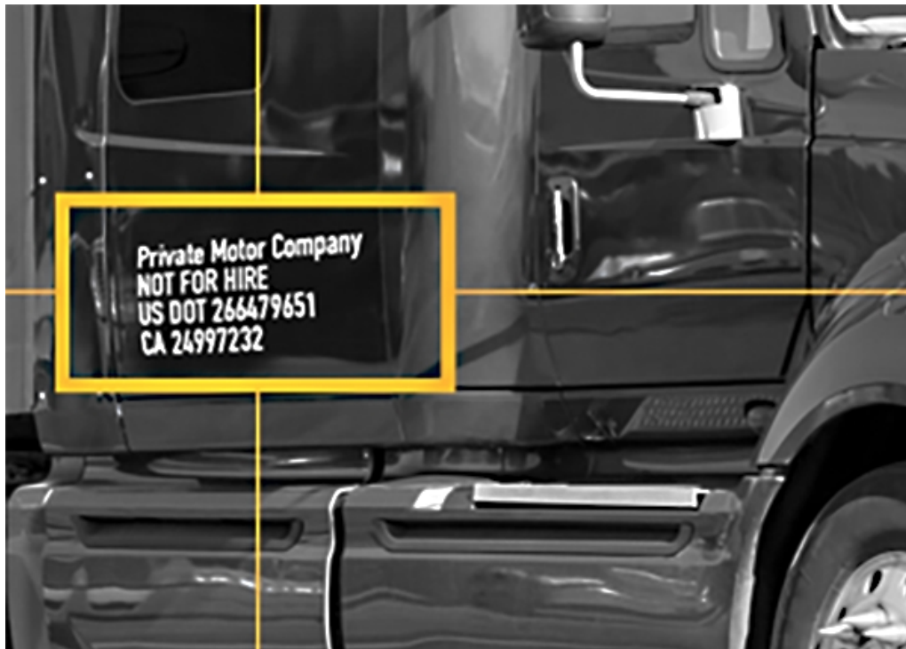
Fig. 17: USDOT code on a truck
