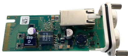
Fig. 4: S74 Network Slide in Board with RJ45 socket
