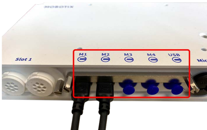
Fig. 22: 4 Module Connector Ports and 1 USB-C interface
