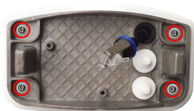
Fig. 6: Installed and ready for Connector Box RJ45
