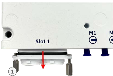
Fig. 18: Remove cover from interface board slot
