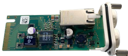
Fig. 4 : S74 Network Slide in Board with RJ45 socket
