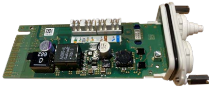
Fig. 7 : S74 Network Slide in Board with LSA terminal
