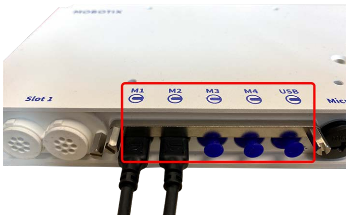
Fig. 4: 4 Module Connector Ports and 1 USB-C interface
