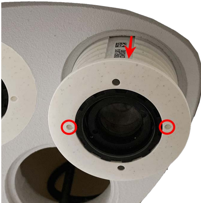
Fig. 10: Remove sensor module from the module housing
