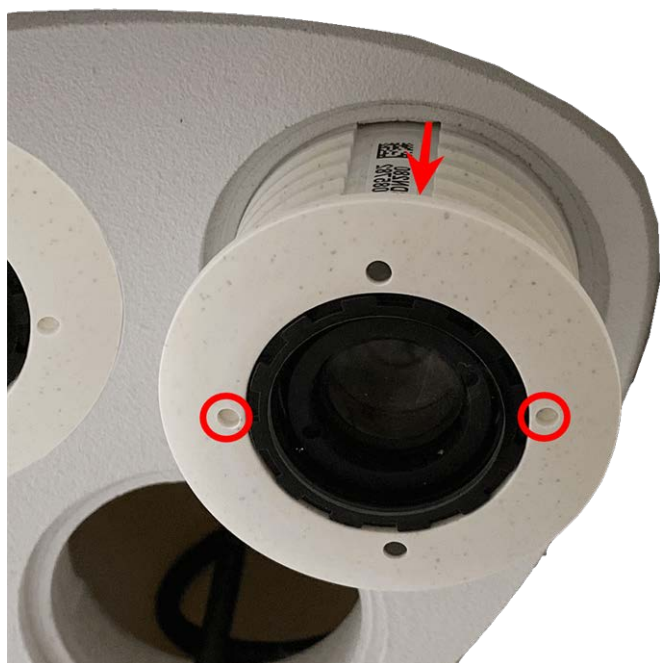
Fig. 10: Remove sensor module from the module housing
