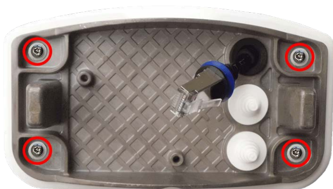
Fig. 6: Installed and ready for Connector Box RJ45
