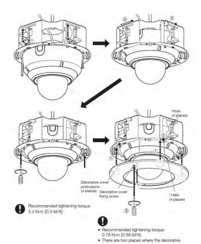
cover fixing screw can be fixed: the position shown in the illustration and the opposite side.
