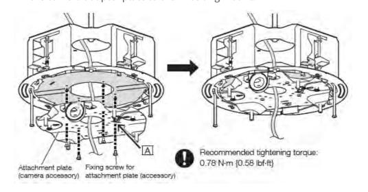
**STEP 9**Mount the camera to the In-ceiling mount.
