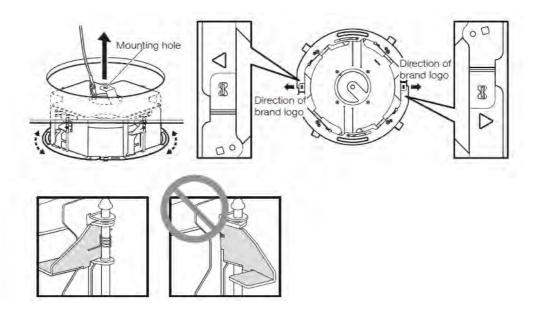
**STEP 6**Secure the mounting chassis.
