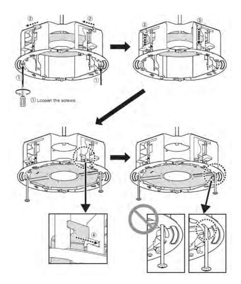
**STEP 8**Fix the camera adapter plate to the In-ceiling mount.
