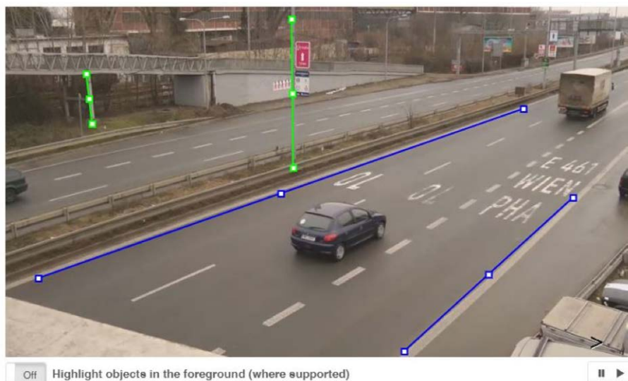
Fig. 89: Draw vertical lines to define the road
