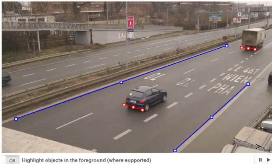
Fig. 91: Draw crossroad lines to define the road
